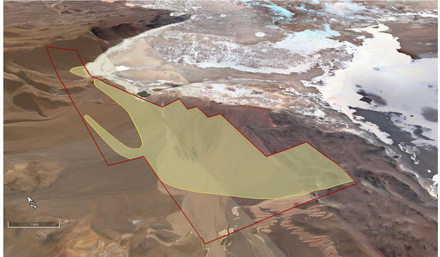
Rincon W property outline in red and surface projection of conductive unit (i.e. potential brines) from TEM survey in yellow
